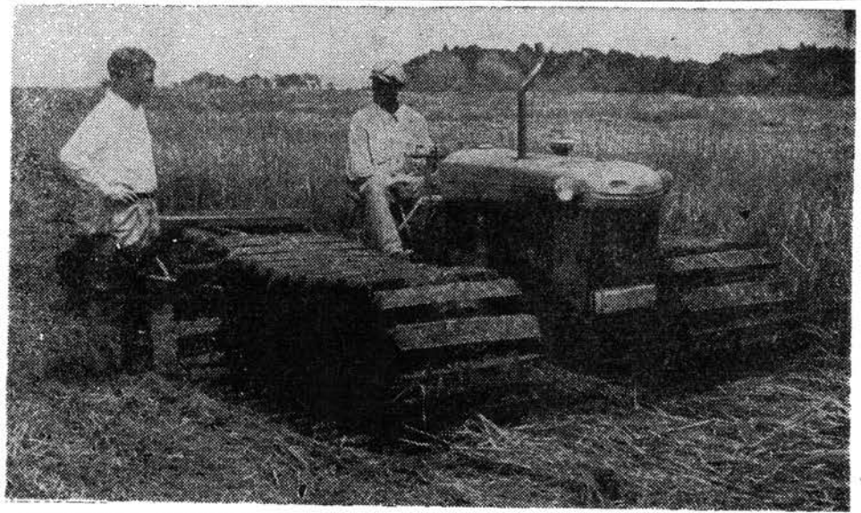
FROM THIS—Andrew H. DuPre, of McClellanville, gives instructions to the operator of his "marsh buggy" on a salt marsh area near McClellanville. The machine, conventional Caterpillar tractor equipped with "out-rider" cleats, operates over marsh areas which barely will support a man walking. Towing a disc-cutter, the buggy chops the salt marsh into the mud, assuring quick rotting when the area is flooded for creation of a duck or fish pond. (Staff Photo by Gilbreth.)
